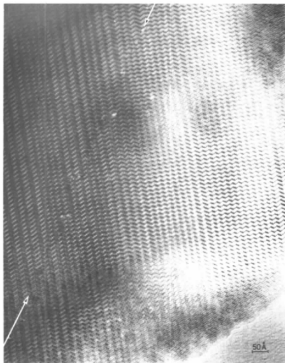
Fig. 14. Electron micrograph of a \text{Mg}_3(\text{Mn}_{2.4}\text{Fe}_{0.6})\text{B}_2\text{O}_{10} crystal with mainly orthopinakiolite structure. The arrows mark a defect boundary where twin slabs of different width meet.
